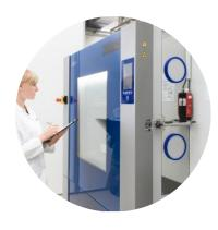
Climatic chambers and shakers integrated into the test station layout as well as safety concept and data acquisition system
