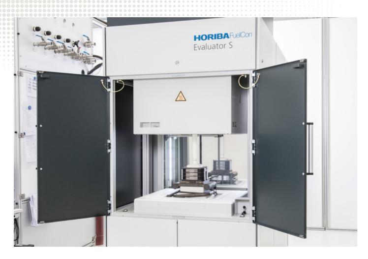
The sintering process includes interconnection of several ceramic MEAs in place to form the SOFC stack. However, this is a crucial task and requires a good amount of precision and reproducibility.
